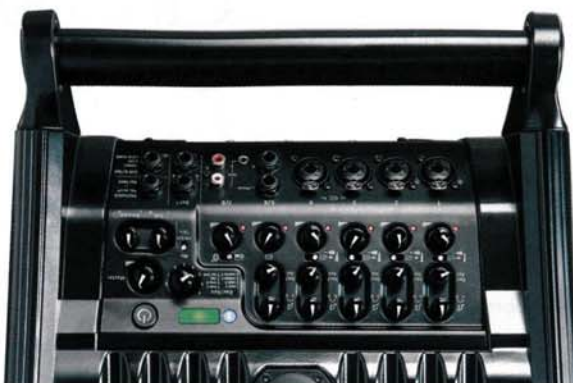
The subwoofer/base unit also houses the system's input connections and controls.
